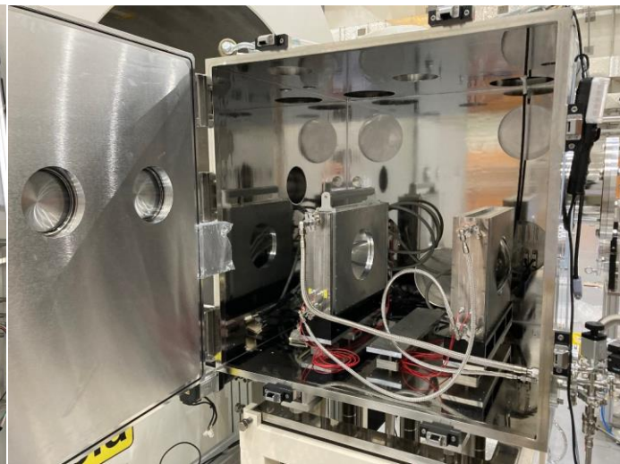
BDC (left) & SC (right) in beam diagnostic vacuum chamber
