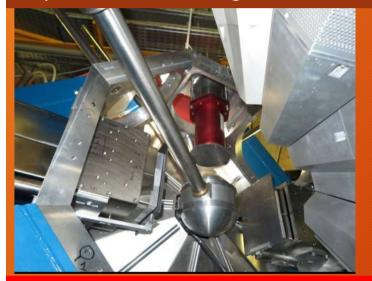
A shield for VAMOS magnetic field needed! Designed at IPHC Strasbourg and tested in dec. 2016 at VAMOS (build of 2 mm mu-metal + 10 mm of mild steel) Additional EXOGAM 3x2mm mu-metal plates
